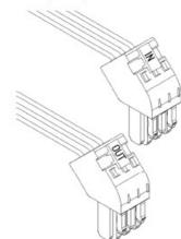
Remove the plugs from the bag and wire the pLAN connections to them. Check the correct orientation of the connections against the terminal labels and wiring diagram. Ensure the other end of the pLAN cable is also correctly terminated.
